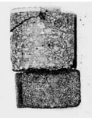
Figure 8: Floor core from Schwelm crew; top carpet, middle mastic asphalt, bottom hard coal/pitch layer
